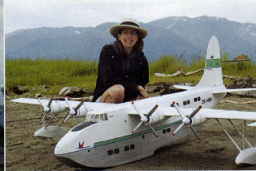
Left: Ivan Pettigrew's all-time favorite flying boat—his scratch-built 100-inch Short Solent—makes a pass along the beach and shows Ivan's piloting skills. This graceful flyer is powered by four Permox 480 motors and has MP-Jet Speed 400 gearboxes. Right: Beverly "Mrs. Tracon" Hudson gives us a sense of scale next to the big boat.
