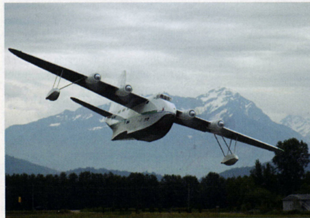
Left: Ivan Pettigrew's all-time favorite flying boat—his scratch-built 100-inch Short Solent—makes a pass along the beach and shows Ivan's piloting skills. This graceful flyer is powered by four Permox 480 motors and has MP-Jet Speed 400 gearboxes. Right: Beverly "Mrs. Tracon" Hudson gives us a sense of scale next to the big boat.
